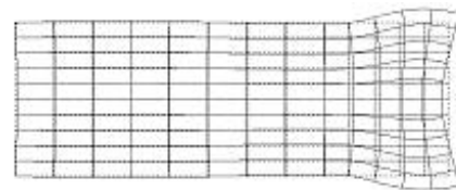
Figure 4 : Displacement field of the PZT5H transducer at 2.5MHz.
