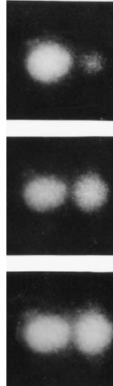
Figure 3: 0 th (left) and 1 st (right) orders of AO diffraction at different levels of acoustic power.
