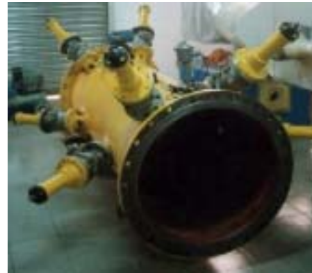
Figure 17: 4 path ultrasonic gas flowmeter
