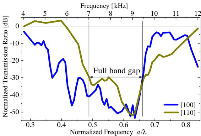
Figure 3: Measured transmission ratio of the sonic-crystal bulk of acrylic resin rods in air.
