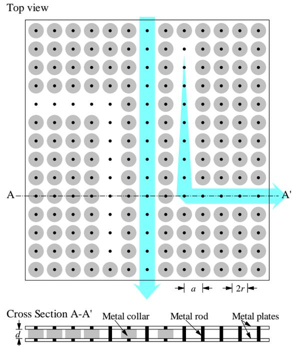
Figure 8: A structure of sonic-crystal slab flexible for sonic circuits.
