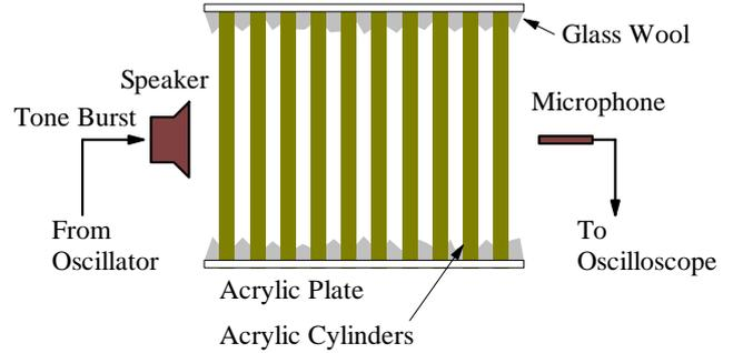
Figure 4: Measurement of the transmission ratio of sonic crystal.
