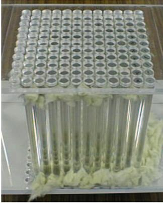
Figure 2: Sonic-crystal bulk of acrylic-resin rods in air.
