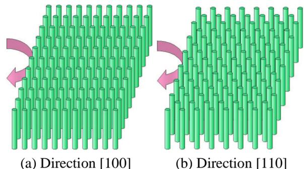
Figure 1: Sonic-crystal. Red arrows show the incident and reflected plane waves.
