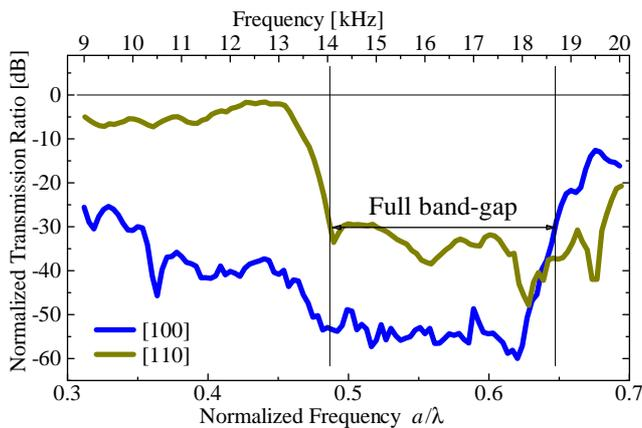
Figure 7: Measured transmission ratio of the sonic-crystal slab.
