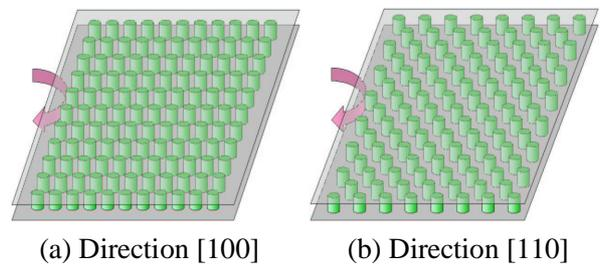
Figure 5: Sonic-crystal slab. Red arrows illustrate the reflected plane waves.
