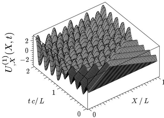
Figure 1: Linear wave profiles superposition evoked by two waves simultaneous propagation.
