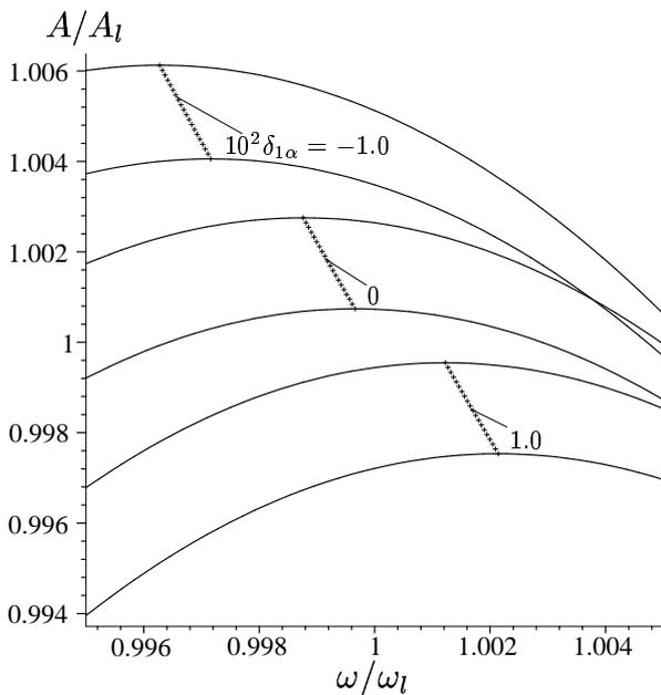
Figure 4: The influence of nonlinearity and physical inhomogeneity on the resonance frequencies.
