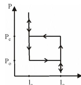
Figure 1 : Rectangular hysteretic mesoscopic elastic unit as used in the PM space model [9]
