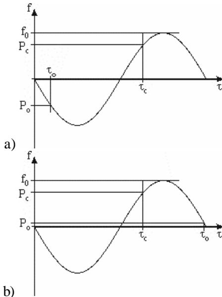
Figure 3 : External sinusoidal excitation  $f(\tau)$ , opening and closing pressures  $P_o$  and  $P_c$  and times  $\tau_o$  and  $\tau_c$  within a cycle are indicated a) starting with a closed and b) starting with an open interface, respectively
