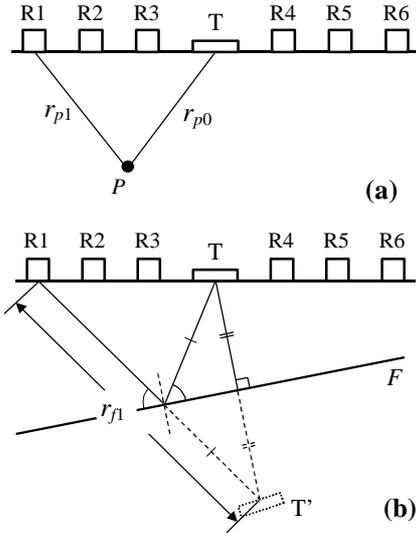
Fig.1 Sound propagating path reflected by (a) underground buried body; (b) underground interface
