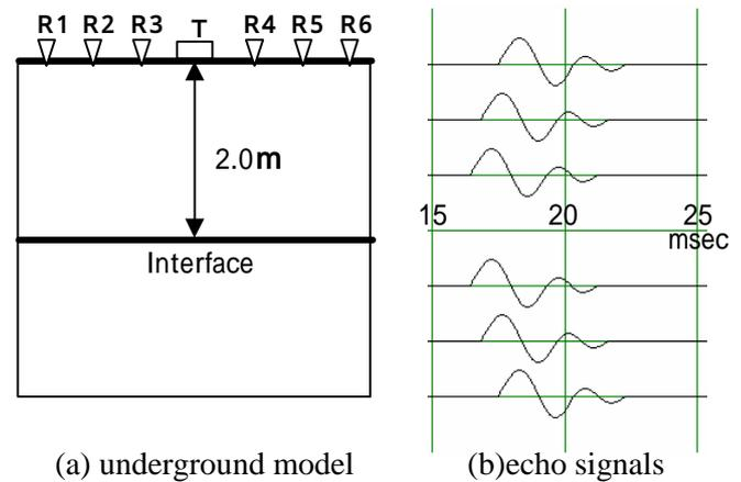
Fig. 4 Simulation model of interface
