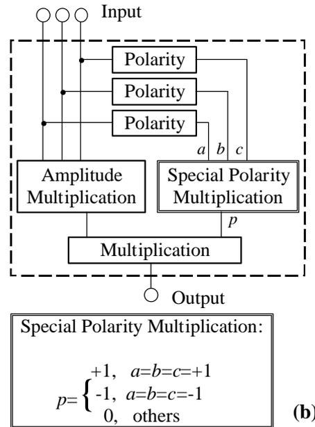
Fig.2 (a) Imaging procedure of ACSP and (b) processing of conditional multiplication
