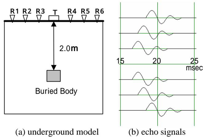
Fig. 3 Simulation model of buried body
