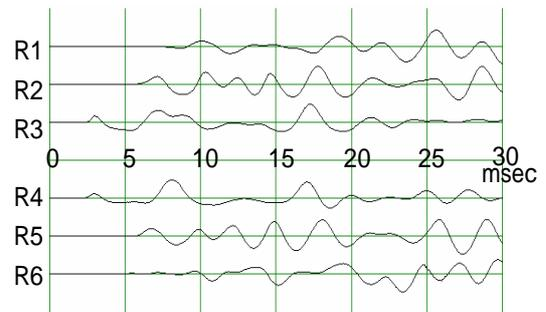
Fig. 8 Example of echo signals from buried body
