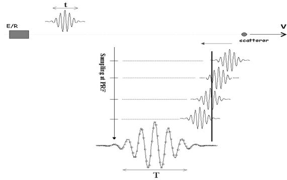
Figure 6: Reconstruction of a Doppler signal through sampling in slow-time timebase
