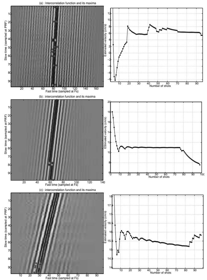
Figure 11: Velocity estimator via intercorelation method for (a):3 l/h, (b):6 l/h and (c):12 l/h flows rates
