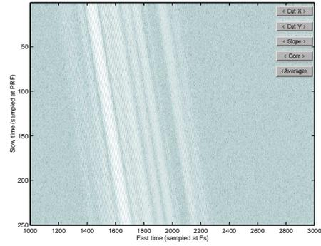
Figure 5: Time  $\times$  time representation of simulated RF lines. (250 shots, SNR=20dB,  $V=5\text{cm/s}$ )
