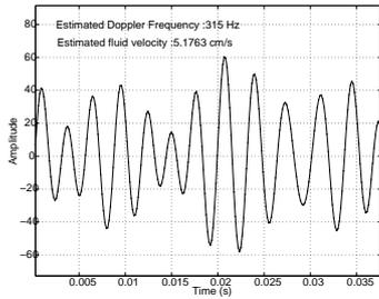
Figure 7: Simulated Doppler signal (10000 particles)
