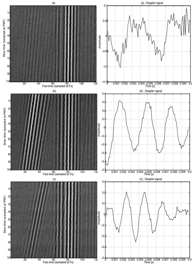
Figure 10: Time-time representations and Doppler signals in the case of 3 l/h (a), 6 l/h (b) and 12 l/h (c) flow rates.
