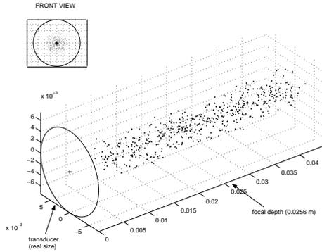
Figure 4: Particles repartition in the simulated sampling volume ( $N_p=500$  particles)
