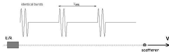
Figure 2: Principle of Pulsed Wave Doppler
