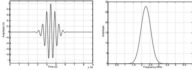
Figure 3: Example of the synthetic emitted pulses and the corresponding spectrum
