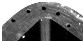
Figure 2: through holes in a radius to be tested externally
