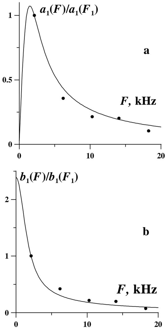
Figure 3 : Experimental (dots) and theoretical dependencies (curves) of parameters  $a_1$  (a) and  $b_1$  (b) on wave frequency  $F_p$
