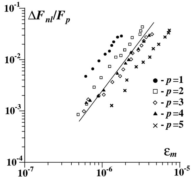
Figure 1 : Nonlinear resonance frequency shift  $\Delta F_{nl} / F_p$  versus wave amplitude  $e_m$  for the five modes of the resonator
