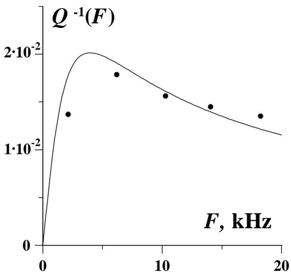
Figure 4 : experimental and theoretical dependencies of  $Q_p^{-1}$  on wave frequency  $F_p$
