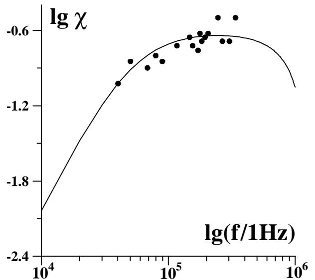
Figure 6 : The dependence of nonlinear damping parameter  $c$  on pulse frequency  $f$
