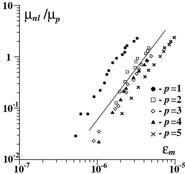
Figure 2 : Nonlinear decrement  $\mu_{nl}$  versus wave amplitude  $\epsilon_m$
