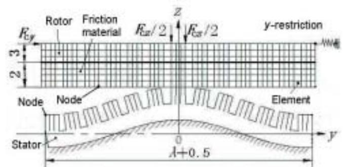
Figure 2 FEM contact model between stator and rotor
