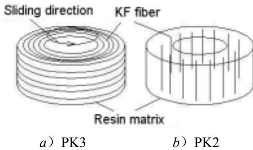
Figure 1 Fiber orientation of friction materials
