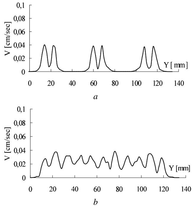
Figure 5. Lateral section of the amplitude of pulsations of the 1-st harmonic of vortex velocity field in the wake past 3 (a) and 10 (b) cylinders for Re=75.
