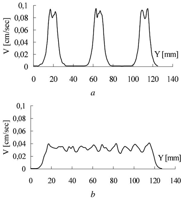
Figure 6. Lateral section of amplitude pulsations of the 1-st harmonic of vortex velocity field in the wake past 3 (a) and 10 (b) cylinders for Re=500.
