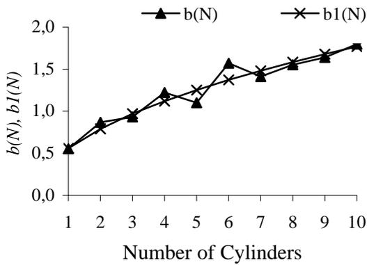
Figure 4. Amplitude of the 1-st harmonic versus number of cylinders for Re=500.
