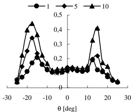
Figure 2. Amplitude of scattering at the +1-st and -1-st harmonics depending on the angle of scattering  $\theta$  for  $Re = 75$  for 1, 5, and 10 cylinders.
