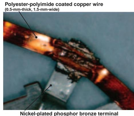
Figure 12: Welded condition of a 0.5-mm-thick, 1.5-mm-wide polyester-polyimide coated flat copper wire and a nickel plated phosphor bronze terminal.
