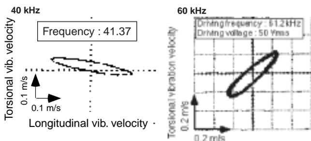
Figure 8: Vibration loci of 40 kHz and 60 kHz complex vibration welding tips at the free edge of the converter. Driving voltage: 50 Vrms.
