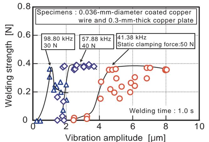
Figure 9: Relationships between vibration amplitude and weld strength of 0.036-mm-diameter coated copper wire specimens using the 40 kHz, 60 kHz and 100 kHz ultrasonic complex vibration welding equipments.
