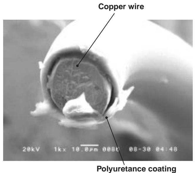
Figure 4. Cross section of 0.036-mm-diameter polyurethane coated copper wire specimen.
