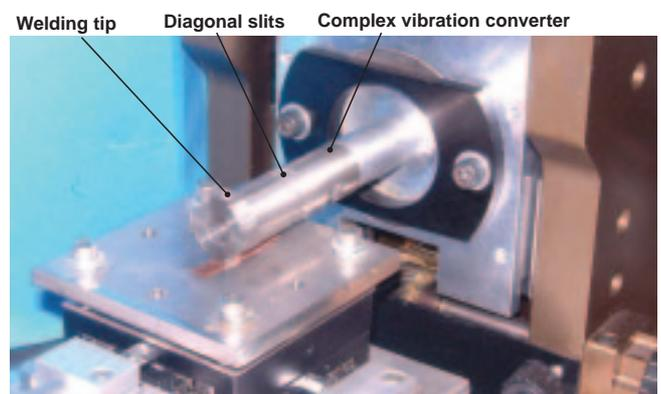
Figure 1: Configuration of a 40 kHz ultrasonic welding system using a longitudinal-torsional vibration converter.
