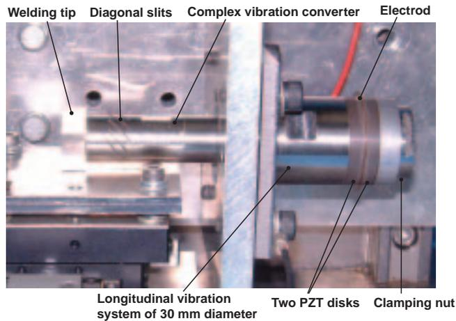
Figure 2: Configuration of a 60 kHz ultrasonic welding system using a longitudinal-torsional vibration converter.
