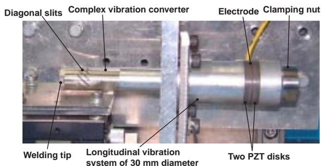
Figure 3: Configuration of a 60 kHz ultrasonic welding system using a longitudinal-torsional vibration converter.
