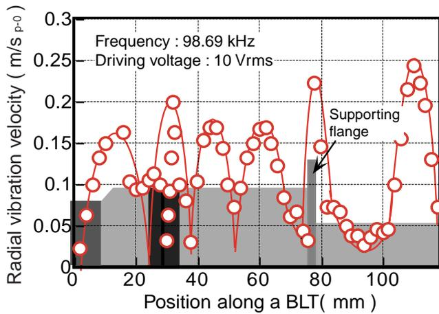
Figure 6: Radial vibration velocity distribution along a 100 kHz longitudinal vibration system of 30 mm diameter with a stepped horn. Driving voltage: 10 Vrms.
