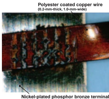
Figure 11: Welded condition of a 0.2-mm-thick, 1.0-mm-wide polyester coated flat copper wire and a nickel plated phosphor bronze terminal.
