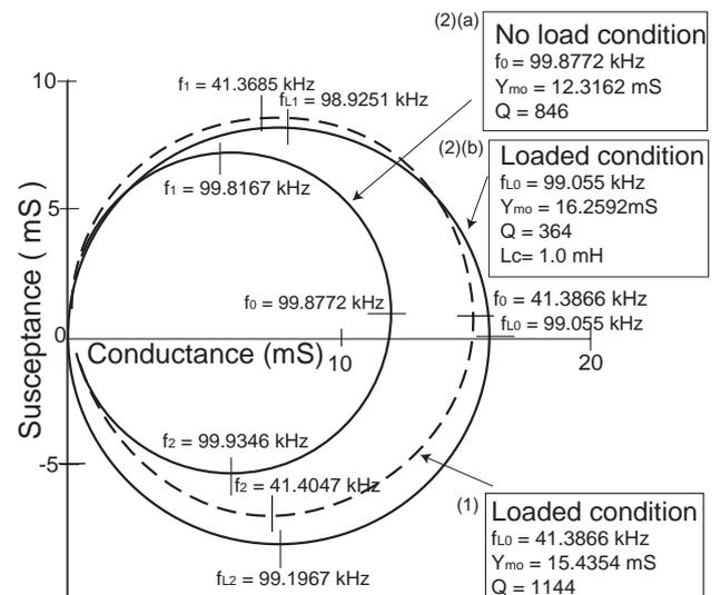
Figure 5: Free admittance loops of (1) a 40 kHz complex vibration system at loaded condition, (2) a 100 kHz complex vibration welding system at (a) no load condition and (b) loaded condition with a power factor compensating inductance.
