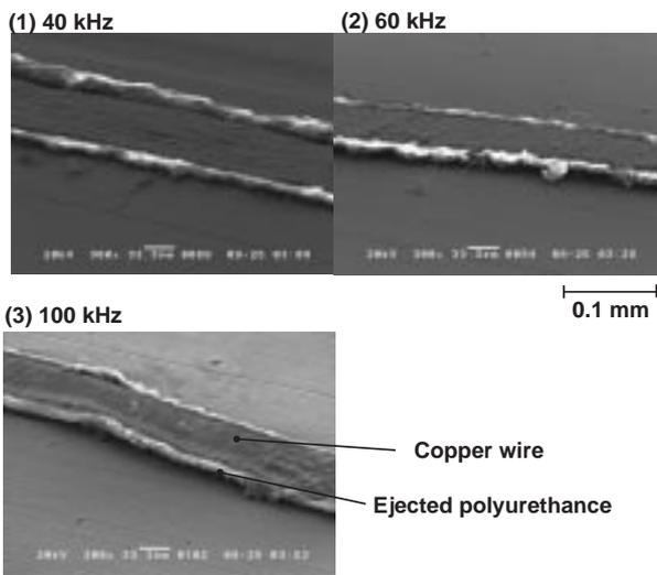
Figure 10: Welded conditions of 0.036-mm-diameter polyurethane coated copper wire specimens joined using by the (1) 40 kHz, (2) 60 kHz and (3) 100 kHz complex vibration welding tip.
