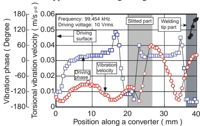
Figure 7: Torsional vibration velocity and vibration phase distributions along a 100 kHz complex vibration converter with a slitted part of 2.0 mm depth. Driving voltage: 10 Vrms.
