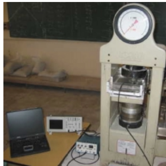
Figure2: General view of the ultrasonic apparatus for evaluating both second (top) and third order elastic constants (bottom).
