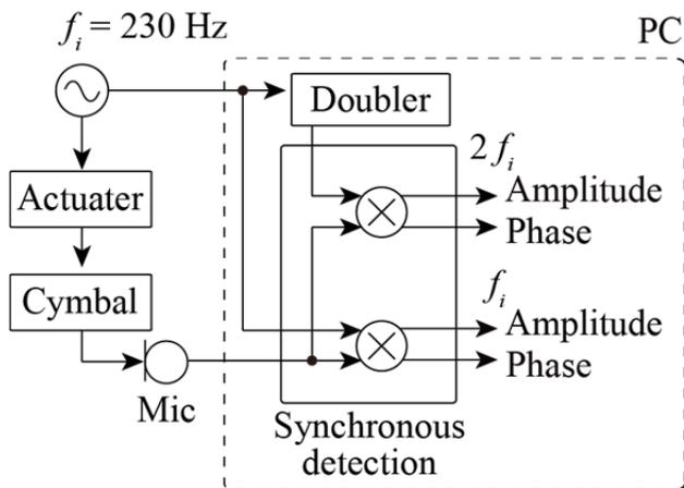
Figure 3: Data flow of Synchronous Detection for extraction of each natural mode.
