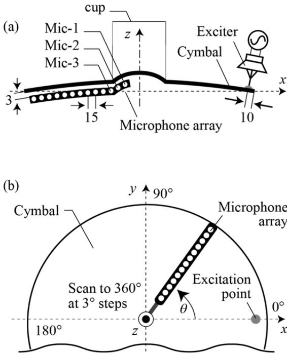
Figure 2: Arrangement of actuator and microphones. (a) Cross section view, and (b) Top view.
