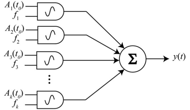
Figure 1: Time varying additive synthesis model for cymbal.
