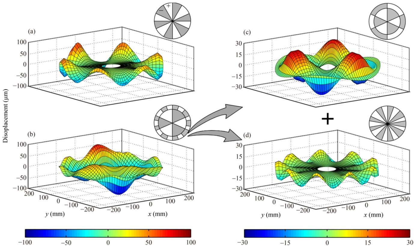
Figure 4: Measured vibrational distribution of amplitude in cymbal. (a)  $f_i$  component which is excited by actuator, and (b)  $2f_i$  component which is excited by inner resonance. (c) (3, 1) mode at natural frequency 455Hz. (d) (9, 0) mode at natural frequency 459 Hz.
