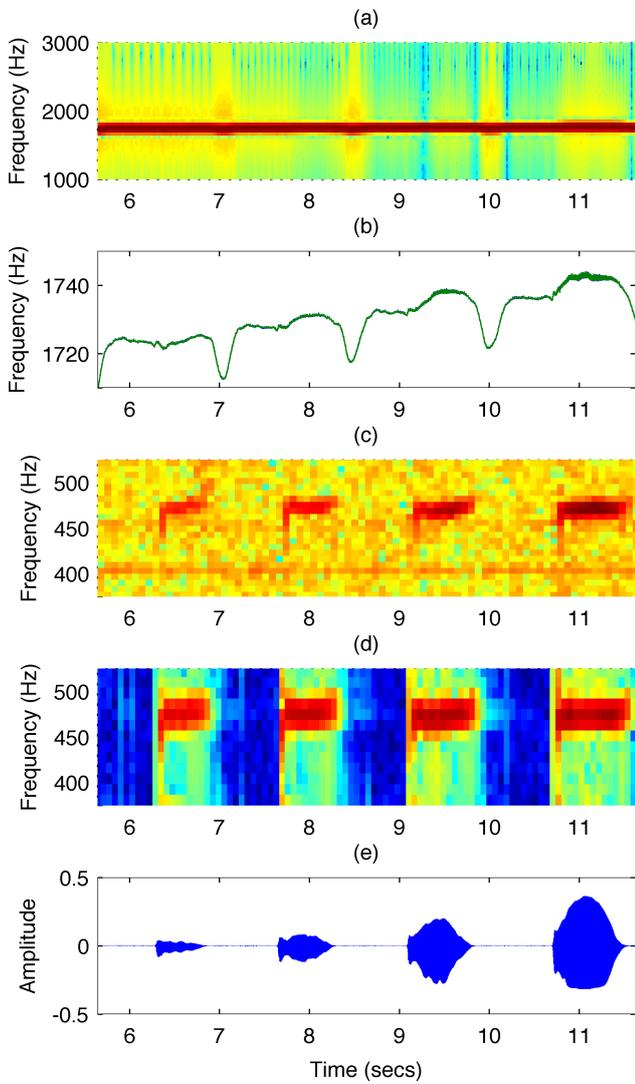
Figure 4: Plots derived for a recording of the note  $Bb_4$  being sounded at different dynamic levels by an experienced jazz player (MV) on the trumpet. (a) Spectrogram of the Theremin output signal. (b) Frequency tracking data calculated from Theremin output signal. (c) Spectrogram of the (high pass filtered) frequency tracking data calculated from the Theremin output signal. (d) Spectrogram of the external microphone signal (e) Audio waveform of the external microphone signal
