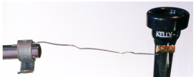
Figure 1: Apparatus (viewed from above) featuring a metal nail with the flat head countersunk on the inside wall of the plastic trumpet mouthpiece and the other end connected to the pitch antenna of a Theremin
