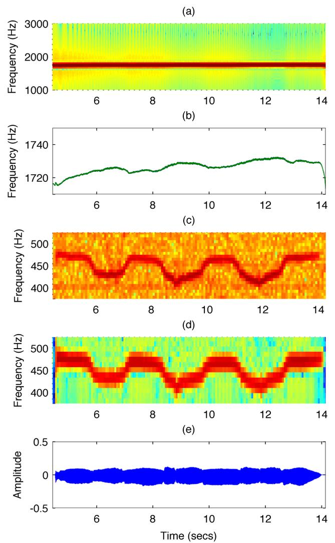
Figure 5: Plots derived for a recording of the note  $Bb_4$  being bent down and upwards in pitch by an experienced jazz player (MV) on the trumpet. (a) Spectrogram of the Theremin output signal. (b) Frequency tracking data calculated from Theremin output signal. (c) Spectrogram of the (high pass filtered) frequency tracking data calculated from the Theremin output signal. (d) Spectrogram of the external microphone signal (e) Audio waveform of the external microphone signal
