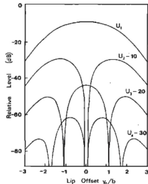
FIG. 3. Calculated relative pressure levels of the first four harmonics in the jet source function as functions of the relative lip displacement  $y_0/b$ , as given by (2). The relative jet displacement amplitude is  $a/b=2$ . For clarity the curves for successive harmonics are displaced downwards by 10, 20, and 30 dB relative to the scale for the first harmonic.
