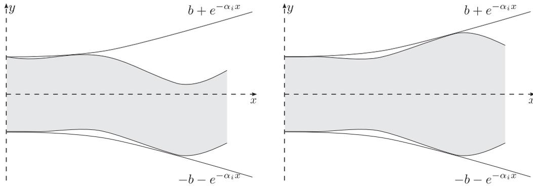
Figure 2: Shapes of the symmetrical (right) and anti-symmetrical (left) unstable modes of jet.
