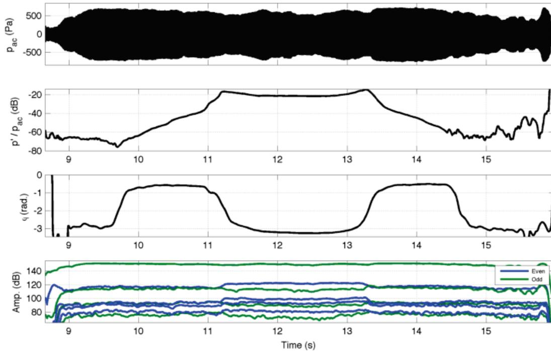
Figure 1: A flautist affirms varying his mouth volume on an isolated note. From top to bottom: internal pressure signal, amplitude of coupling, phase of coupling and strength of the 8 first harmonics of the internal pressure.
