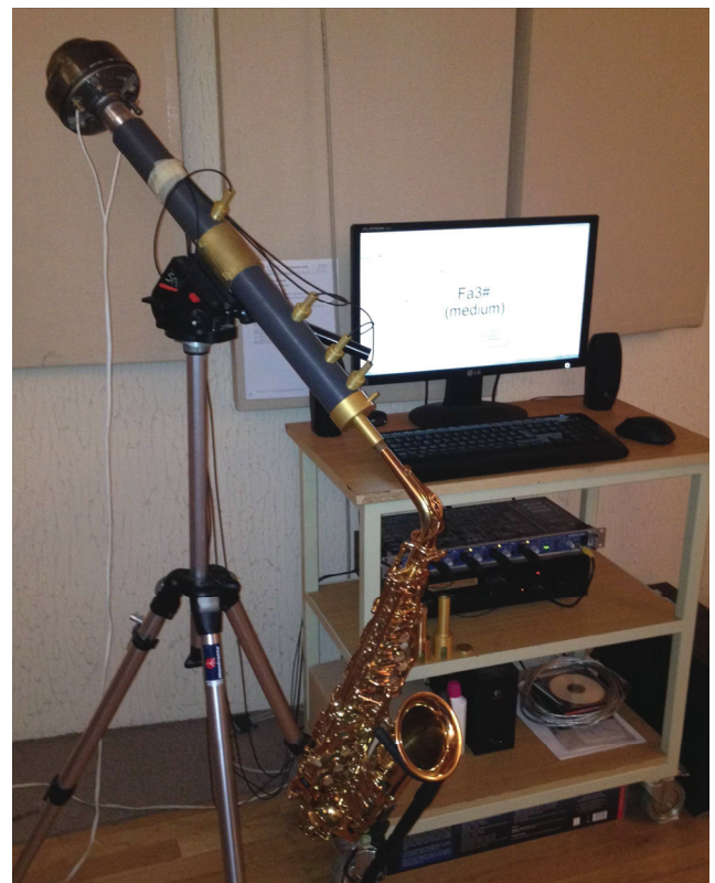
Figure 2: Complete measurement installation with the analysis unit.
