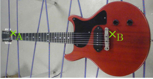
Figure 1: The guitar of the study at stage 6 (fully-equipped guitar). The two crosses indicates the two measurement points: one close the nut (A), the other close to the bridge (B).
