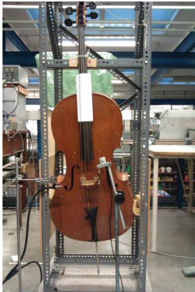
Figure 3: Cello set up for input admittance measurements.
