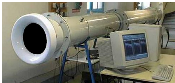
Figure 6: Aeroacoustic test bench of the axial fan.
