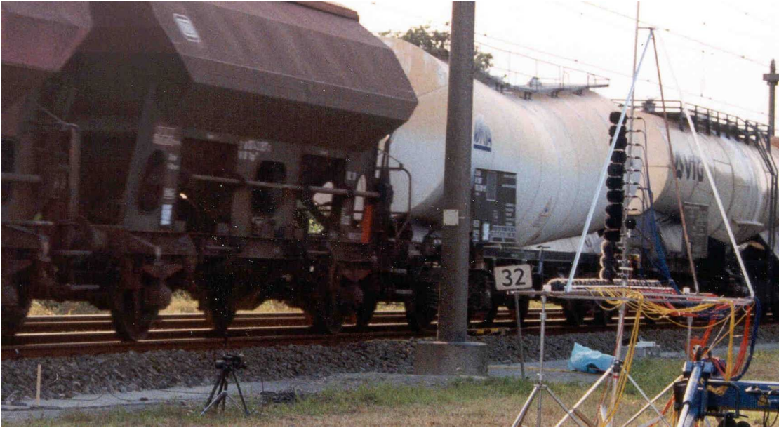
Figure 9: T-array measurement set-up.
