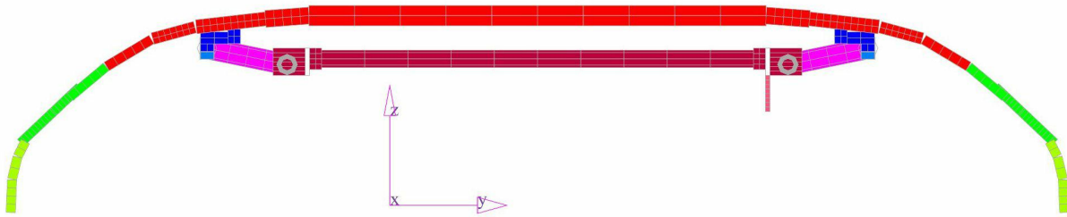
Figure 2: The model of the pantograph ASP (front view); the horn ends are vertical orientated.
