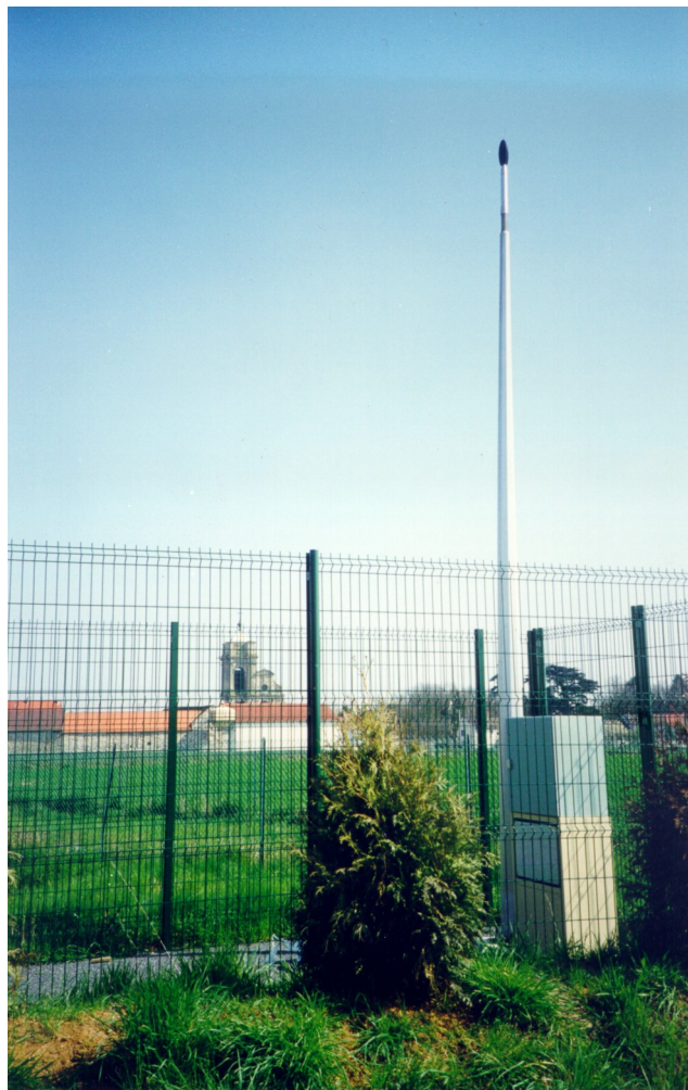
Figure 1: Noise monitoring terminal around CDG.
