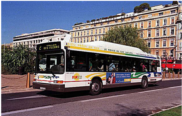
Figure 6: Bus running on natural gas (noise reduction 5 dB(A)).
