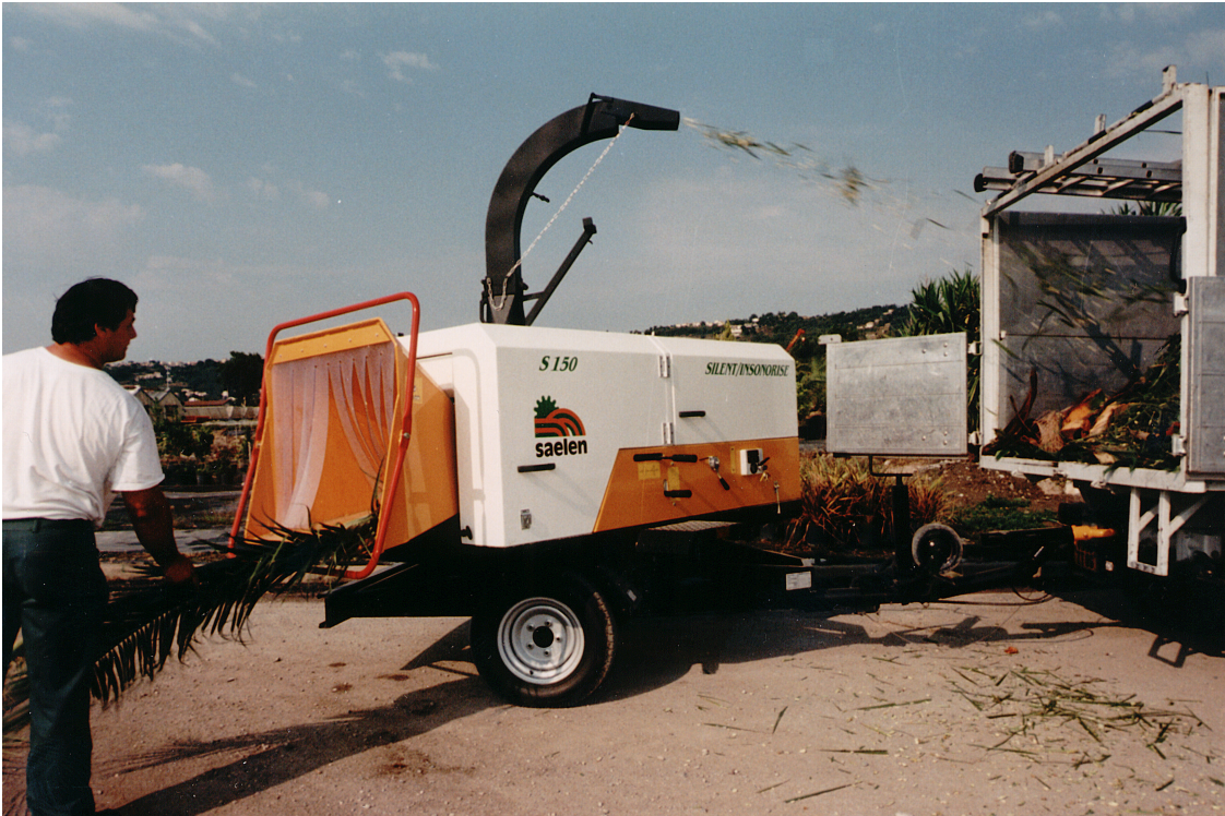
Figure 7: Vegetal shredder (noise reduction 5 dB(A)).
