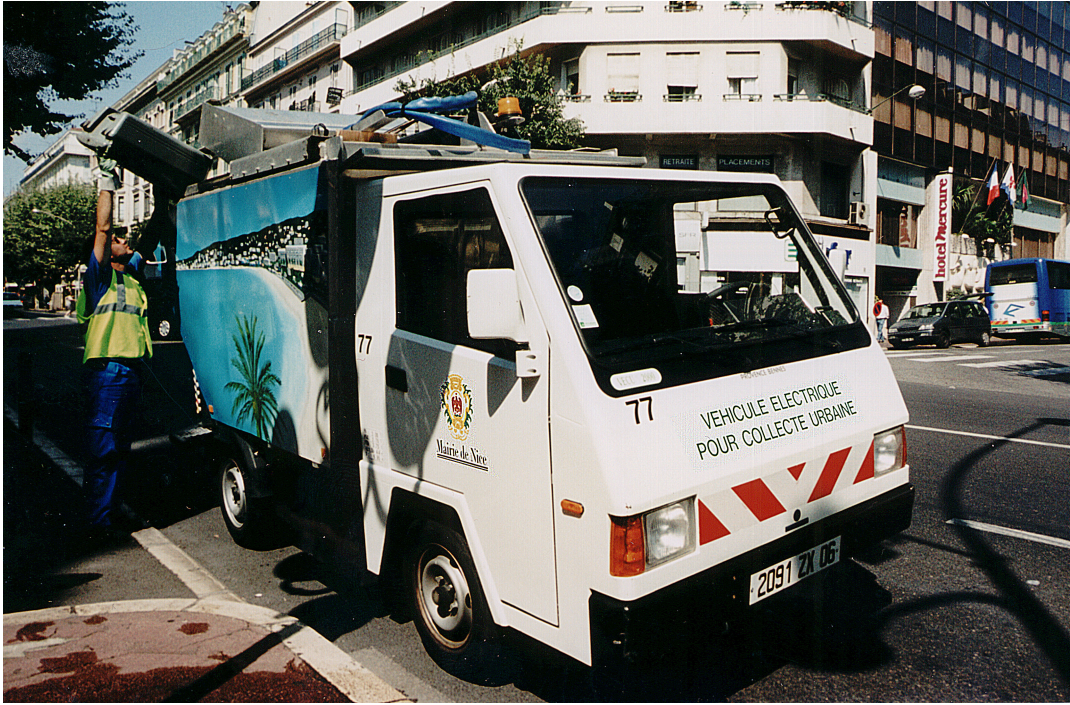
Figure 5: Electric vehicle for refuse transport.
