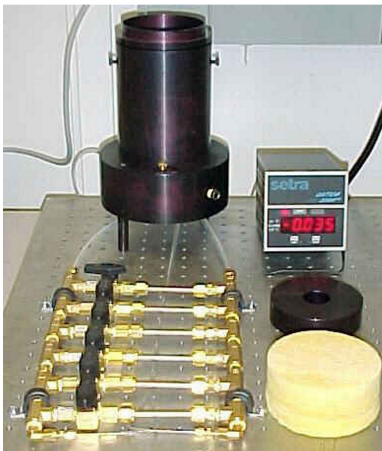
Figure 2: UTRC choked orifice flow resistance tester.
