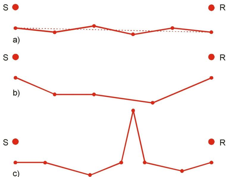
**Figure 1:** Segmented terrain in the propagation model: a) flat terrain b) valley-shaped terrain c) hill-shaped terrain.
