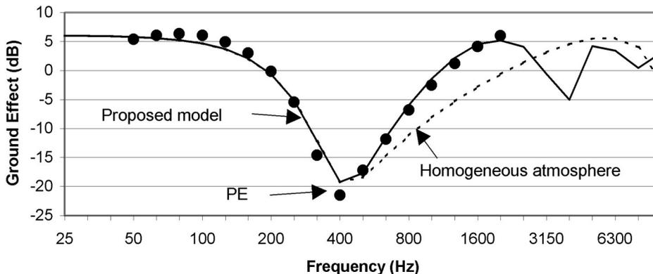
**Figure 3:** Ground effect over flat grass-covered terrain predicted by the proposed model and by PE in a downward refracting atmosphere;  $d = 200$  m,  $h_S = 2$  m,  $h_R = 1.5$  m, wind speed at 10 m = 1 m/s.
