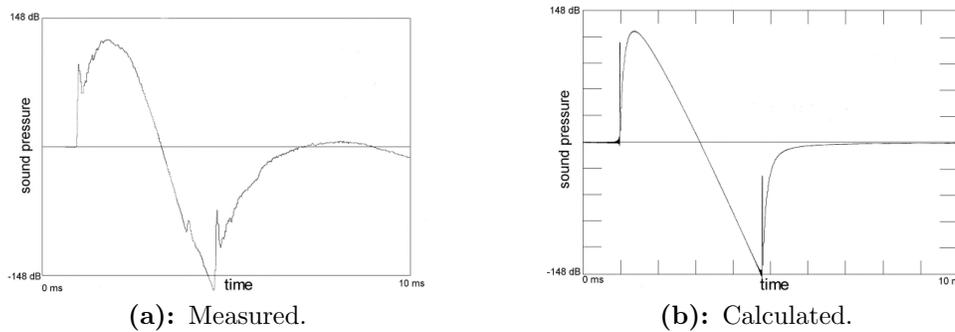
**Figure 1:** Sound pressure versus time for sonic boom from a howitzer shot at  $r = 88$  m distance and 0 m height.
