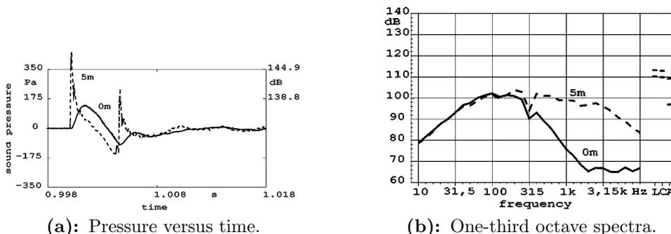
**Figure 2:** Sonic boom from a howitzer shot measured at  $r = 122$  m at 5 m (solid lines) and 0 m (dashed lines) height.
