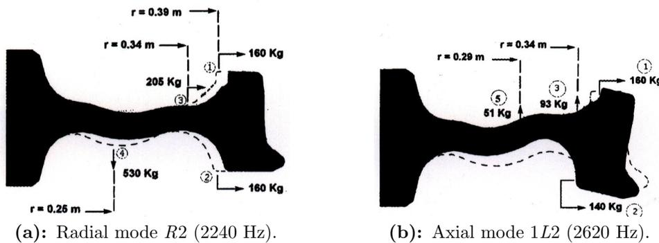
**Figure 2:** Apparent modal mass at specific point on wheel.
