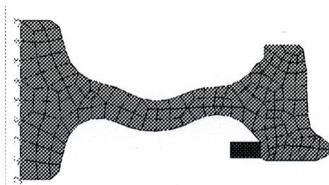
**Figure 3:** Axisymmetric mesh of the wheel with one set of dynamic absorber, tuned at a single frequency (not to scale).
