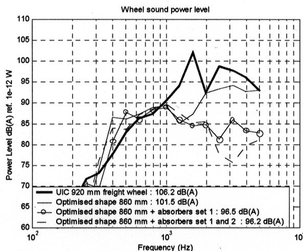
Figure 4: Sound power radiated by one wheel, at 100 km/h (dB(A), calculation).
