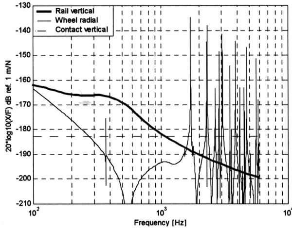
**Figure 1:** Track, wheel and contact receptances at wheel/rail interface; vertical direction; freight configuration (UIC60 rail with twin bloc sleepers and ballast, freight wheel).
