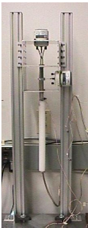
Figure 5: Experimental rig for measuring tortuosity, viscous and thermal characteristic lengths and elastic moduli (cylindrical sample is melamine foam).
