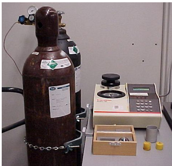
Figure 2: Flow resistivity and porosity experimental rigs.
