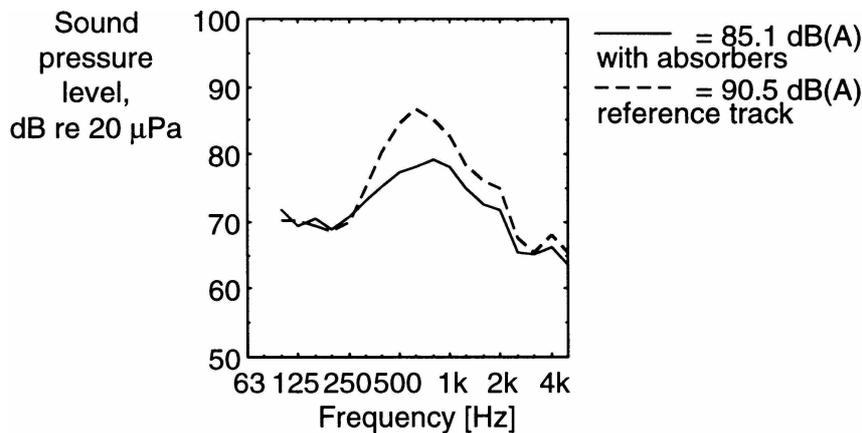
**Figure 6:** Results of measurements of rolling noise at 100 km/h using a vehicle fitted with a noise reducing wheel. Average from three microphones at 3 m from near rail.
