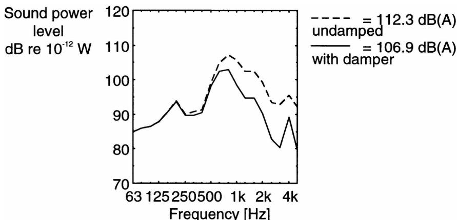
Figure 5: Predicted rail sound power with and without the absorbers.
