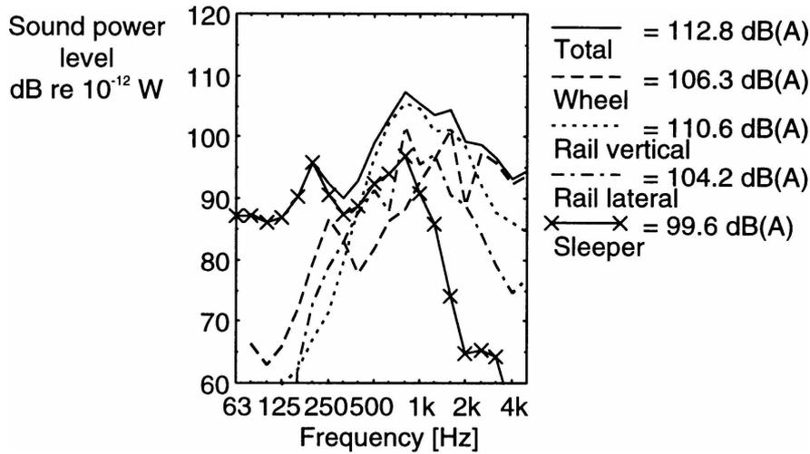
**Figure 1:** Predicted rolling sound power generated per wheel for a standard 920 mm freight wheel running on a standard track at 100 km/h.
