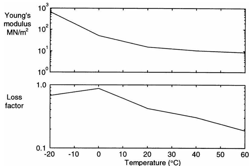
**Figure 3:** The temperature dependent Young's modulus and loss factor of the elastomer.
