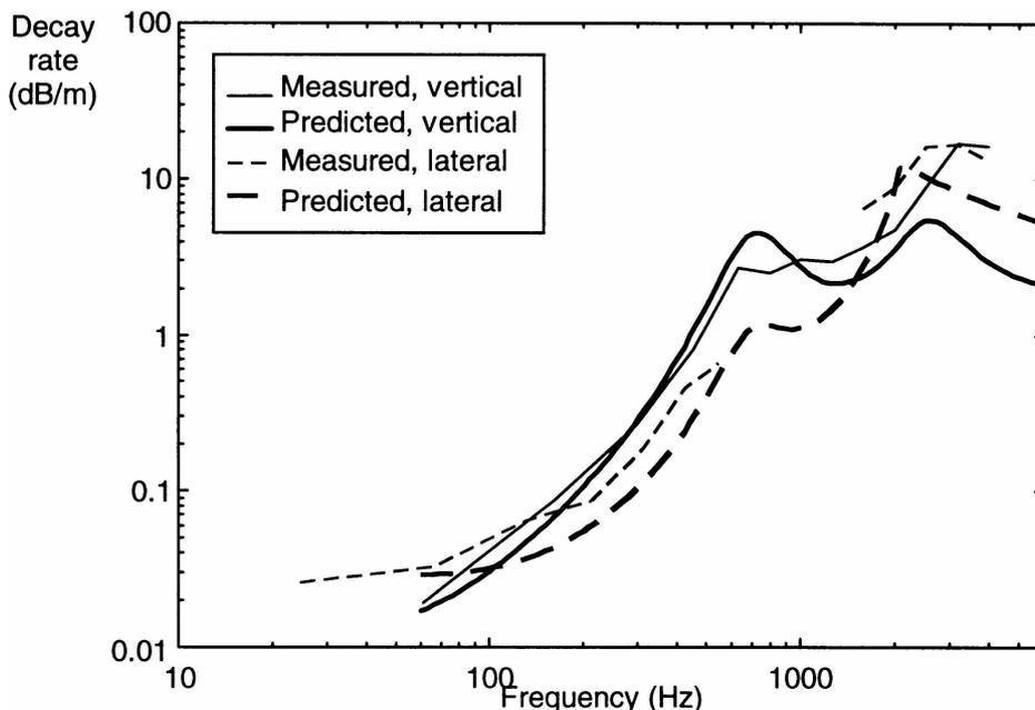
Figure 4: Predicted decay rates compared to measurements on a 4 m long freely suspended rail.
