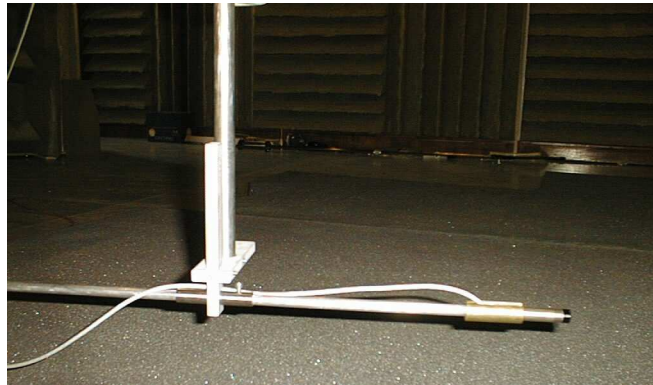
Figure 2: Detail of distance probe.
