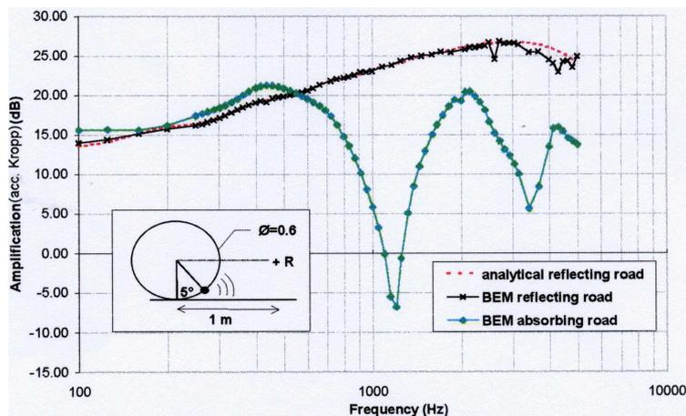
Figure 2: Comparison 2D analytical / 2D BEM and effect of absorption on the road.
