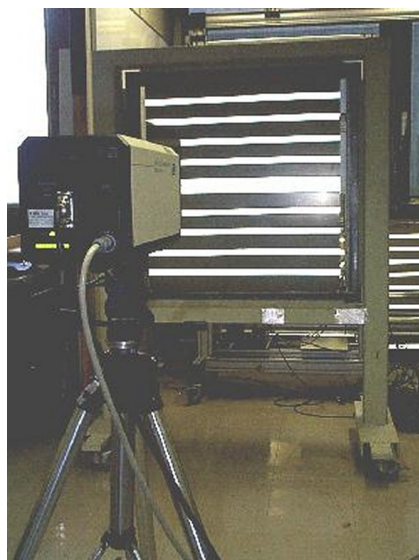
Figure 2(c): Experimental set-up for technique of scanning laser vibrometry.
