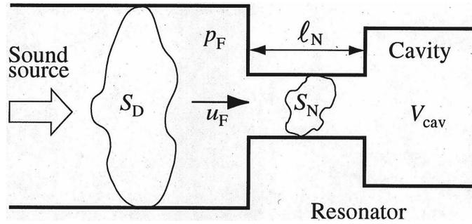
Figure 1: A Helmholtz resonator at an end of a straight duct.
