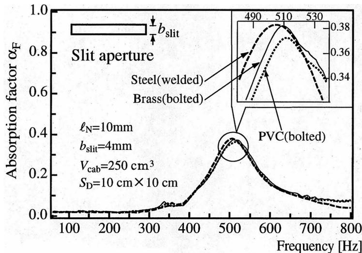
Figure 2: Dependence of the absorption factor on materials.
