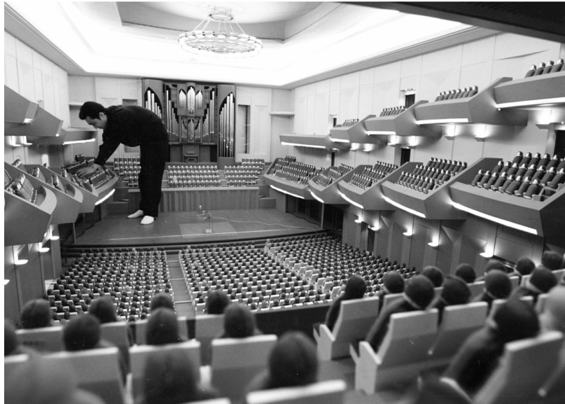
Figure 6: 1/10 scale model experiment for acoustic design of concert hall.
