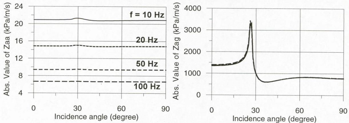
**Figure 1:** Variation with incident angle of absolute values of  $Z_{aa}$  and  $Z_{ag}$  for  $V_s = 300$  m/s.
