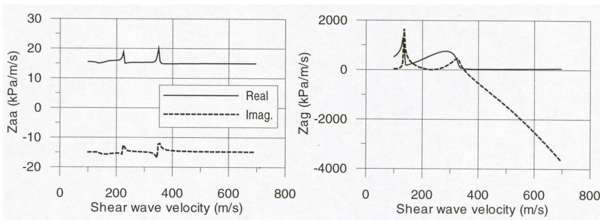
**Figure 2:** Variations of real and imaginary parts of  $Z_{aa}$  and  $Z_{ag}$  with  $V_s$  for  $f = 10$  Hz.
