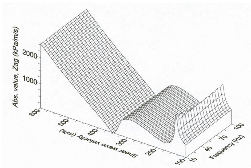
Figure 3: Variation with frequency and shear-wave velocity of absolute value of  $Z_{ag}$ .
