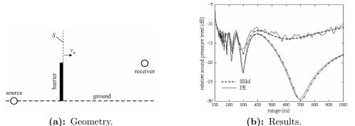
Figure 1: The two upper curves show the sound field behind the barrier for a turbulent atmosphere using SSM and PE; the two lower curves are for a non-turbulent situation.
