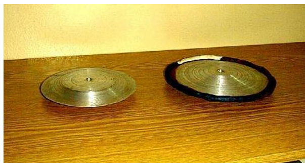
Figure 5: Tapered disk (the right disk is coated with the plasticine around the border).
