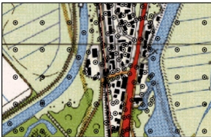
Figure 3: Density of observation points is dependent upon the variation in noise levels.
