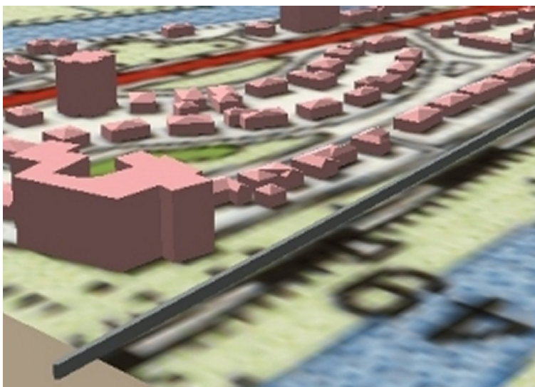
Figure 2: An example of using a 3D data-model of buildings in generating noise data-models.
