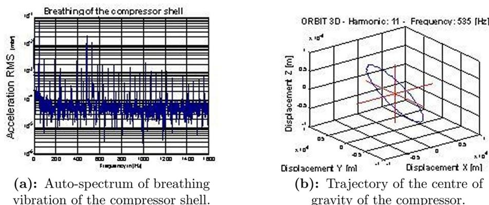
(a): Auto-spectrum of breathing vibration of the compressor shell.
