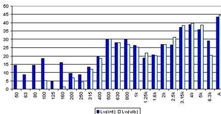
**Figure 3:** Sound power level radiated by a refrigerant compressor; dark columns – results obtained using the intensity measurement; light columns – results obtained using the vibration measurements and the computation procedure described in the paper.
