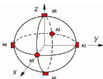
(a): Schematic presentation of 6 accelerometers antenna/array.
