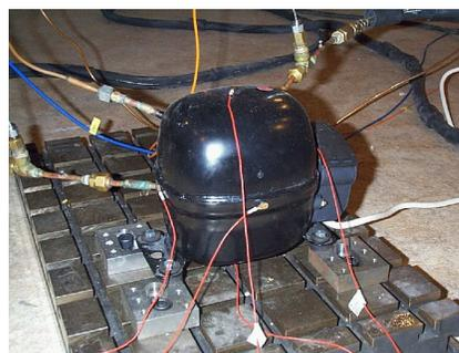
(b): Measurement antenna/array applied to a small refrigerant compressor.
