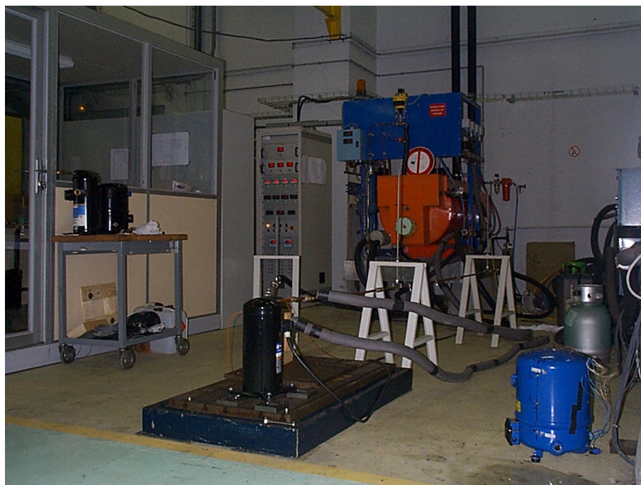
Figure 1: The test-rig for vibroacoustic characterisation of refrigerant compressors under controlled operating conditions.
