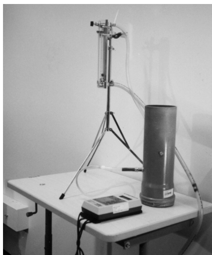
Figure 1(a): The constructed airflow resistance measurement tube.
