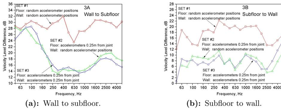
**Figure 3:** Measured velocity level difference in the two directions using different accelerometer positions.
