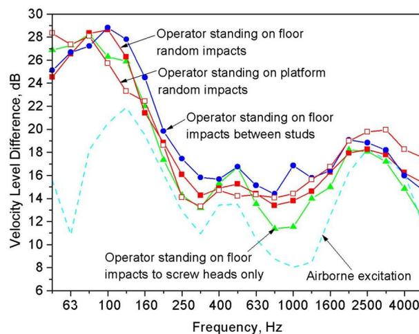
**Figure 2:** Measured velocity level difference between a gypsum board wall and the subfloor as a function of different excitation methods; the accelerometer positions were the same for all measurements.
