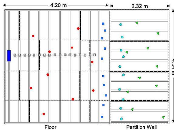
**Figure 1:** Accelerometer locations for the measurement of VLD between the subfloor and wall are shown by the solid symbols; also shown by the open symbol are the positions used for the draw-away measurements on the floor.
