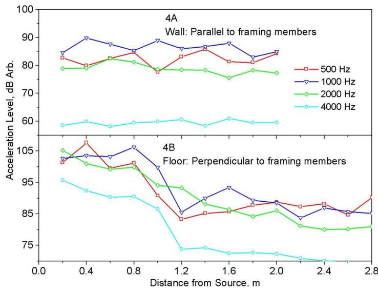
**Figure 4:** Measured surface velocity as a function of distance from the source for the gypsum board wall and the wood joist floor; the captions in the top right-hand corners indicate the surface and the direction of propagation with respect to the framing members.
