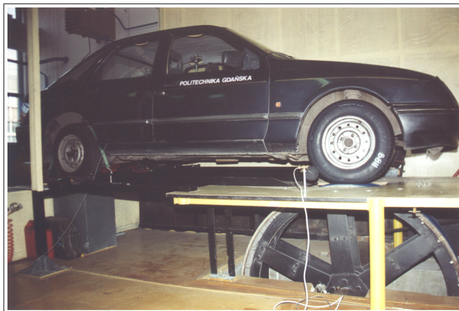
Figure 1: Test car on the roadwheel facility at the Technical University of Gdansk.
