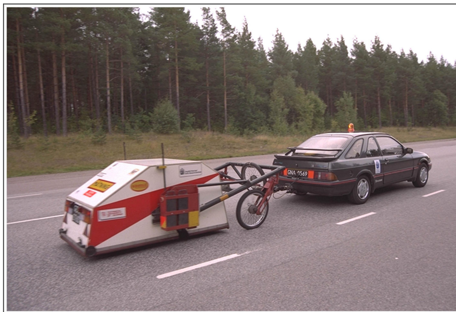
Figure 2: Test trailer "Tiresonic Mk 2" built at the Technical University of Gdansk, Poland.
