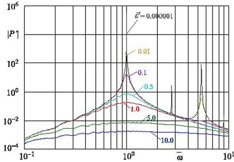
**Figure 1:** The normalized total sound power modulus of an annular plate  $|P'|$ , where  $s=1.2$ ,  $h=1e-3m$ .
