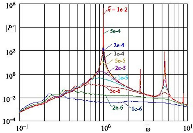
**Figure 2:** The normalized total sound power modulus of an annular plate  $|P'|$ , where  $s=1.2$ ,  $\varepsilon'=1e-6$ , the plate's thickness  $h$  is the curve parameter.
