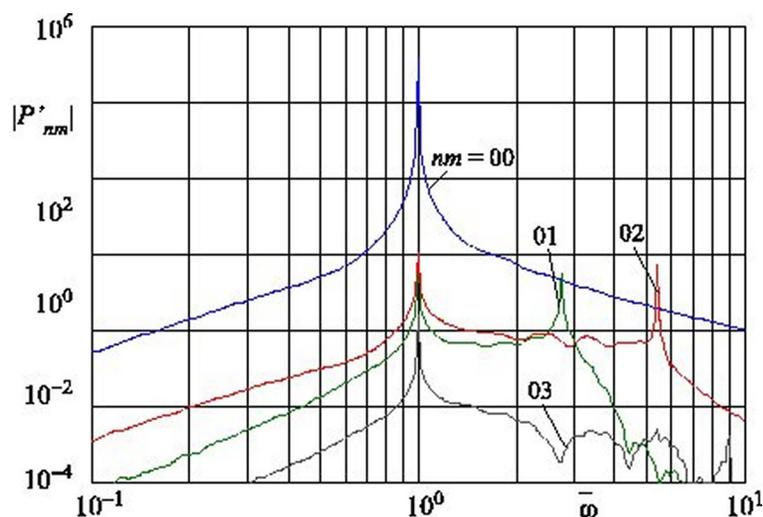
Figure 3: The mutual sound power modulus  $|P'_{nm}|$ , where  $s=2$ ,  $h=1e-3m$ ,  $nm=00, 01, 02, 03$ .
