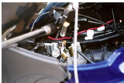
Figure 2: The set-up for the near field noise and injector surface vibration measurements for S2.
