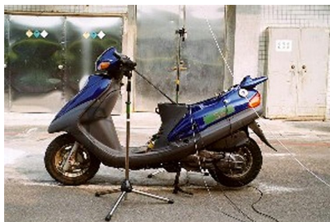
Figure 1: The set-up for the far field and near field noise measurements for S2.
