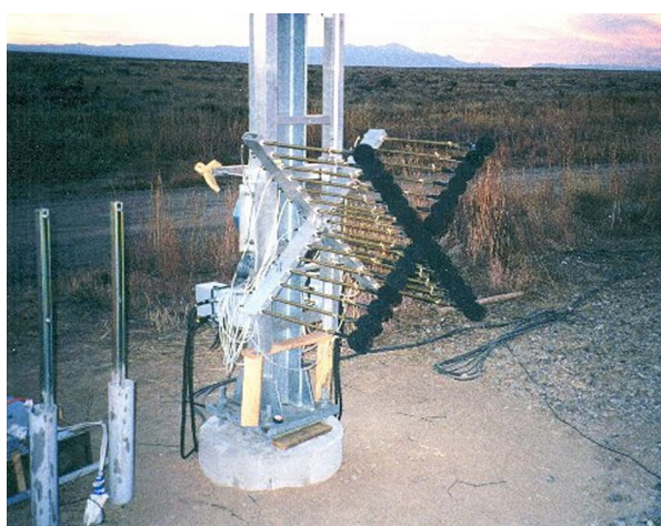
Figure 2: Example microphone array for Acela diagnostic tests at TTC.
