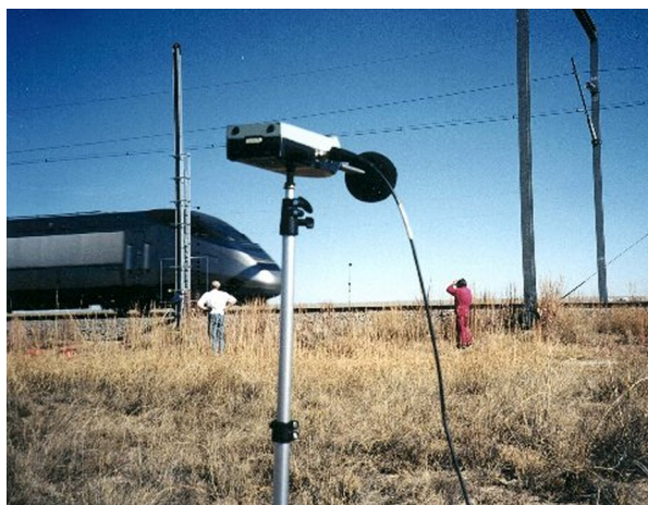
Figure 1: Single point microphone for emission compliance.
