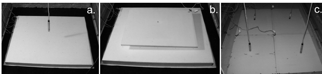
Figure 2: Location of the sensors and the actuators: a. – single sensor (microphone) and single actuator; b. – distributed sensor (EMF panel) and single actuator; c. – 4 sensors (microphones) and 4 actuators.
